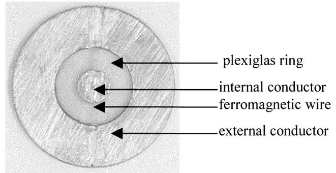
Fig. 4. Coaxial line sample of wire composites.
