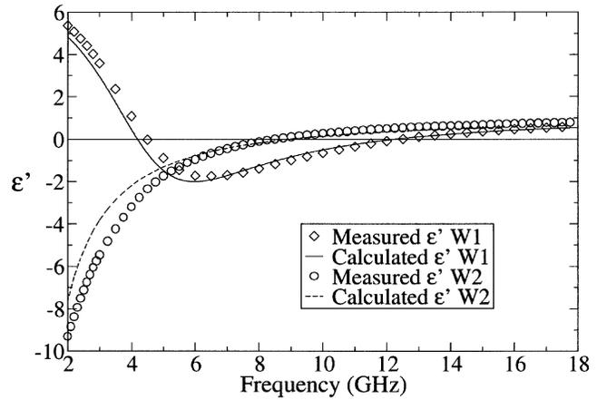
Fig. 5. Measured and calculated real part of the effective permittivity of a lattice of microwires W1 and W2.
