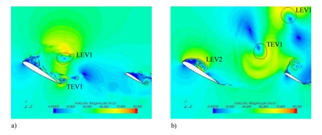
**Figure 1.** Velocity magnitude and identification of vortices with the *Q*-criterion (black line) for: a) minimum value of tail lift. b) maximum value of tail lift. LEV1: leading edge vortex 1, TEV1: trailing edge vortex 1, LEV2: leading edge vortex 2.
