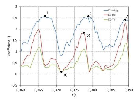
Figure 2. Time development of wing (blue) and tail (red) lift coefficients and tail (green) drag coefficent: a) minimum value of tail lift, b) maximum value of tail lift.
