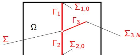
Figure 1: Example of a 2D domain  $\Omega$  and 3 intersecting fractures  $\Gamma_i$ ,  $i = 1, 2, 3$ .
