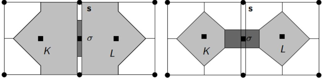
Figure 3: For VAG-1 (left) and VAG-2 (right), example of the choices of the control volumes at cells, fracture face, and nodes, in the case of two cells  $K$  and  $L$  splitted by one fracture face  $\sigma$  (the width of the fracture has been enlarged in this figure).
