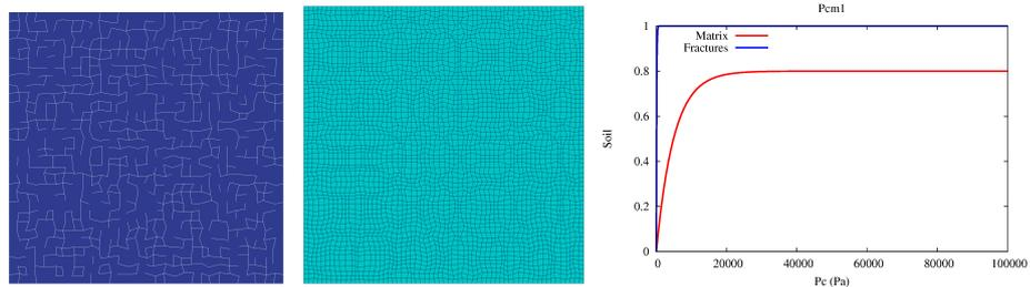
Figure 7: Network of 927 fractures and mesh obtained for  $n_x = 60$ . Inverses of the extended monotone graphs of the capillary pressures  $S_m^1$  in the matrix, and  $S_f^1$  in the fractures.
