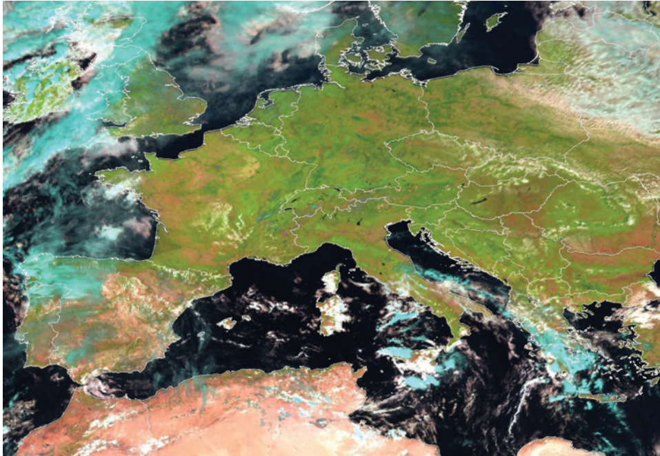
Europe as observed from a geostationary satellite (RGB composition of MSG-SEVIRI data, 22 Sep 2010): red and green show land and vegetation, respectively, while white and blue show thick and cold clouds, respectively. (Courtesy of F. Olesen, KIT)
