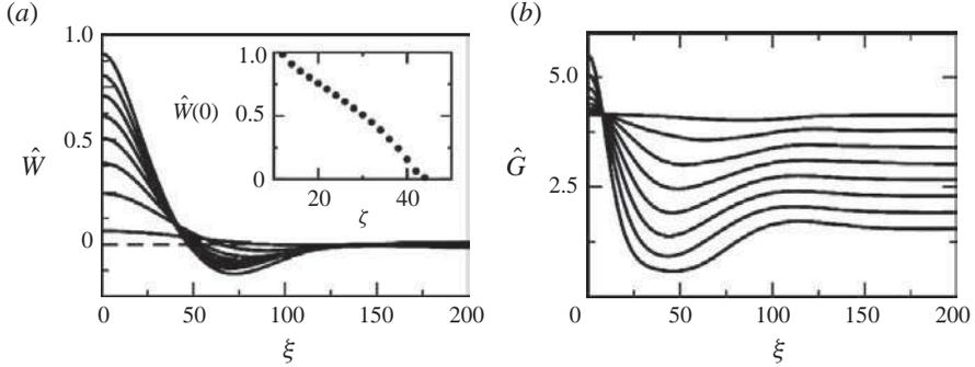
FIGURE 3. Variation of plume properties at equally spaced depths. (a) Vertical velocity  $\hat{w}$  and (b)  $\hat{G}$ , the total reduced gravity, for the parameters defined in table 1, at  $\zeta = 14, 18, 22, \dots, 42$ . The inset of (a) shows the downward velocity at the centre of the plume as a function of depth.
