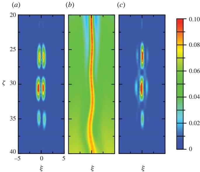
FIGURE 10. Spatial dependence of contributions to power balance for the sinuous instability. Localization of regions of (a) strong buoyancy flux contribution and (c) dissipation at time  $\tau = 83.67$  compared with the total reduced gravity field  $\tilde{G}$  at time  $\tau = 133.67$  shown in (b).
