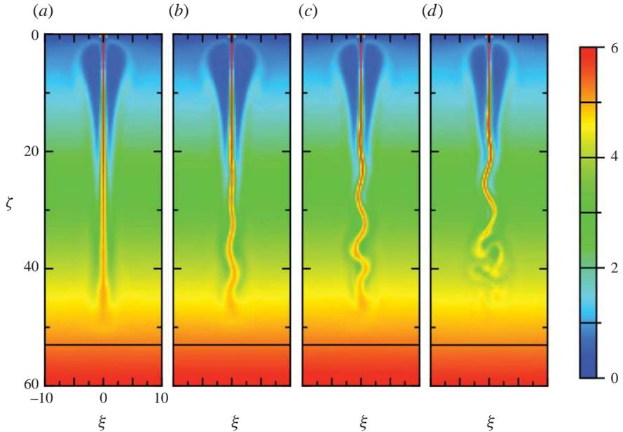
FIGURE 8. Development of the sinuous instability. Results for  $Re_{in}=0.05$ ,  $Sc=667$  and  $Gr=49.05$  for (a) the base flow and  $\tau =$  (b) 133.67, (c) 200.33 and (d) 250.33. The horizontal black line marks the penetration depth for the equivalent base plume flow.
