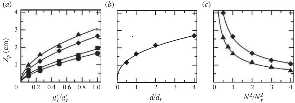
FIGURE 4. Variation of penetration depth with flow parameters, at  $Pe = 0$ , for (a) relative source reduced gravity  $g'_i/g'_r$ , (b) relative source width  $d/d_r$  and (c) relative dimensional buoyancy frequency  $N^2/N_r^2$ , where the reference values are as defined in table 1. Numerical results are marked with the symbols, and the best-fit power laws are shown with the solid lines.
