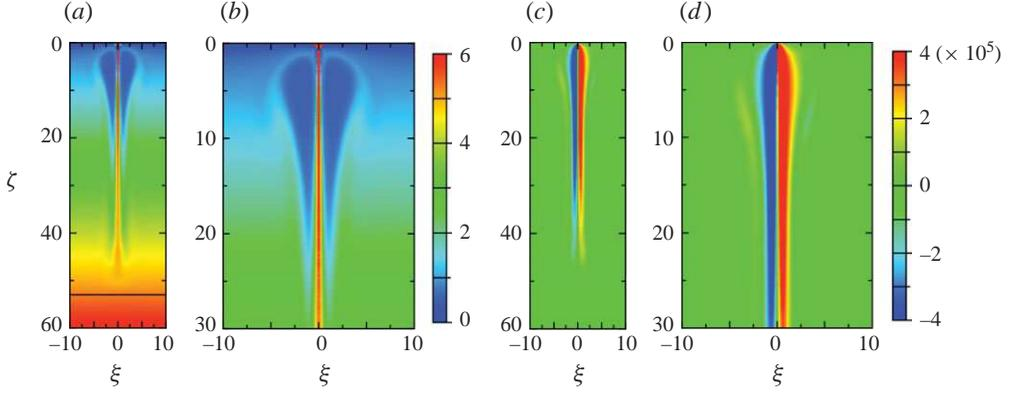
FIGURE 2. The reference base plume flow as defined in table 1. (a) Total reduced gravity  $\hat{G}$  as defined in (2.6) and (b) enlargement of source region. (c) Vorticity  $\hat{\Omega}$  and (d) enlargement. The black line in (a) marks the penetration depth.
