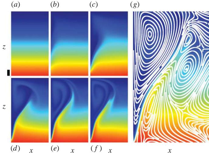
FIGURE 5. Moving-wall simulations. (a)–(f) Evolution of the total reduced gravity at times  $t=0, 100, 300, 600, 1000$  and  $1200$  s after the start of the motion. (g) As shown by the white streamlines, the conduit of fresh water displays a sharp edge that coincides with the separatrix between the large vortex adjacent to the wall and the remainder of the flow. The scale bar is 2 cm.
