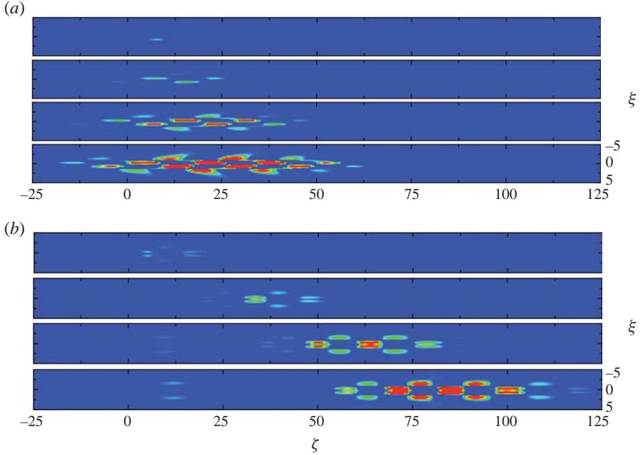
FIGURE 11. Plots of perturbation reduced gravity  $\tilde{g}$  as defined in (2.10) for a ‘reference case’ linearized flow with the parameters as given in table 1 and  $Re = 0.05$  in a parallel flow with vertical velocity and steady reduced gravity ( $g_s$  as in (2.10)) fields extracted from a base flow plume at height  $\zeta_s = 16$  for times  $\tau = 13.33, 46.67, 80$  and  $106.67$  after the initial perturbation for (a) sinuous and (b) varicose perturbations.
