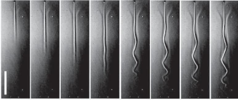
FIGURE 1. Descent of a saline jet into a salinity gradient. Schlieren images at injection rates from  $0.02$  to  $0.18 \text{ cm s}^{-1}$  into a gradient with a buoyancy frequency  $N = 1.5 \text{ s}^{-1}$ . The scale bar is  $1 \text{ cm}$ . Image adapted from Pesci, Porter & Goldstein (2003).
