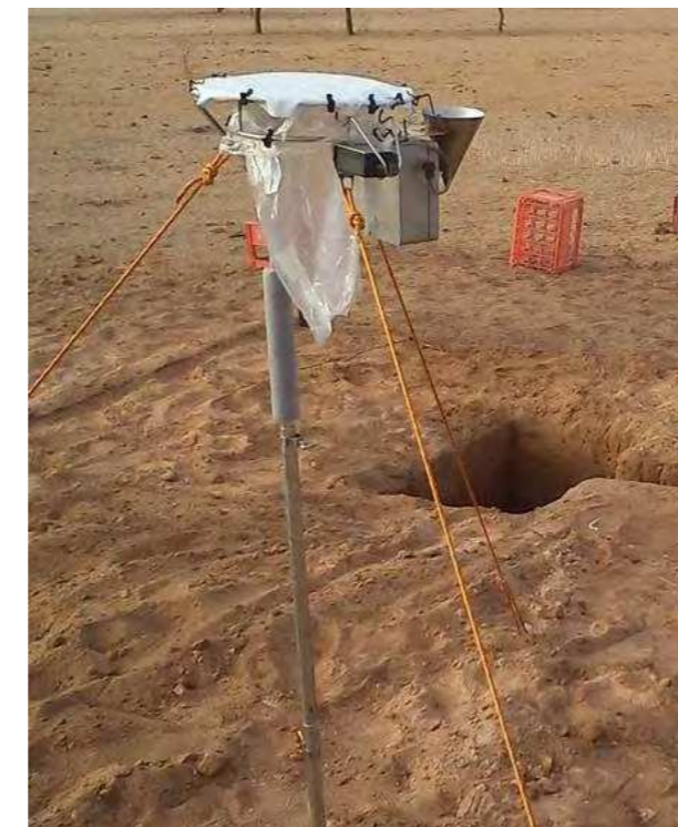
Rain collector => NH 4 + and NO 3 - concentrations in rain
