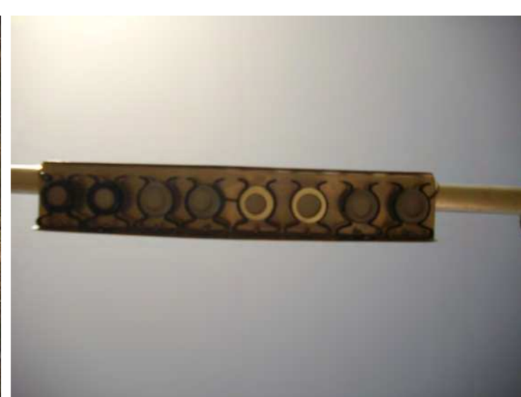
Passive samplers => NH 3 , NO 2 , HNO 3 , O 3 ambient concentration.
