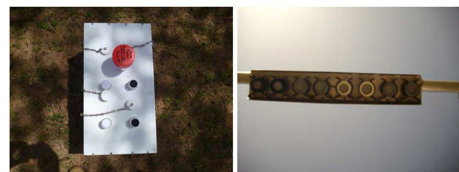
Teflon chamber: Passive samplers => NH 3 volatilization from animal excreta
