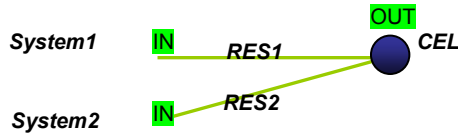
Figure 6. Subtraction of system output signals using the GENESIS symbolism
