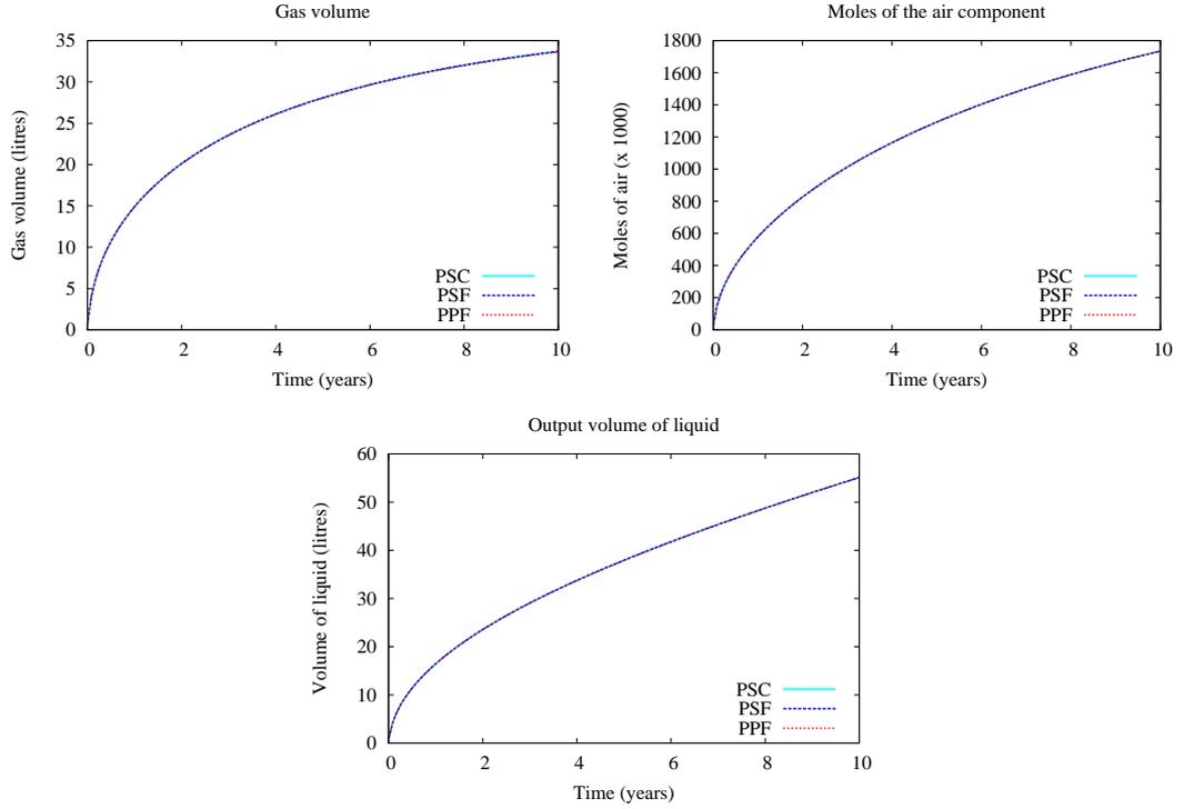
Figure 5: Comparison of the gas volume, the number of moles of the air component, and the output volume of liquid at time  $t = 10$  years obtained with the mesh  $N = 27$  and the three formulations PPF, PSF and PSC.
