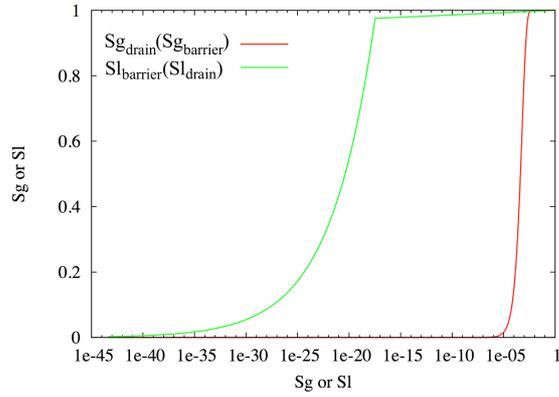
Figure 13:  $S_{drain}^g = 1 - P_{c,drain}^{-1}(P_{c,barrier}(1 - S_{barrier}^g))$  function of  $S_{barrier}^g$  and  $S_{barrier}^l = P_{c,barrier}^{-1}(P_{c,drain}(S_{drain}^l))$  function of  $S_{drain}^l$ .
