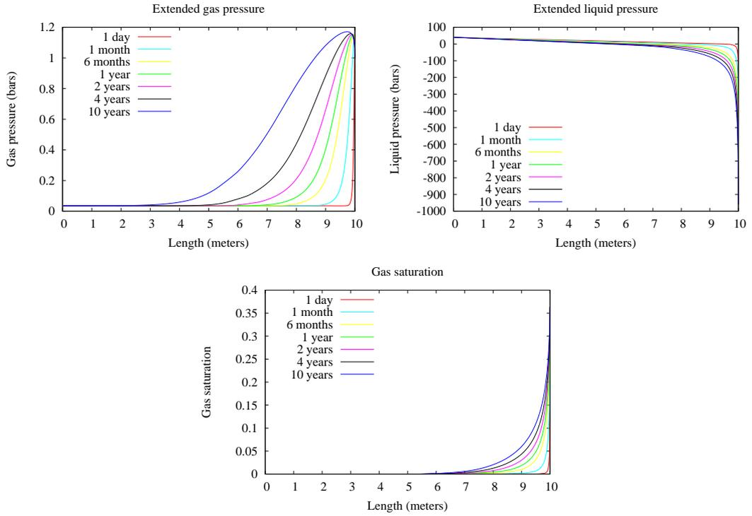
Figure 2: Gas saturation, and extended gas and liquid pressures  $\tilde{P}^g$ ,  $\tilde{P}^l$  at times  $t = 1$  day, 1 month, 6 months, 1 year, 2 years, 4 years, and 10 years obtained with the mesh  $N = 559$  and the PPF formulation.
