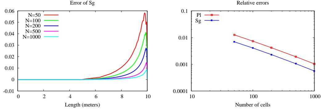
Figure 6: Convergence of the discrete gas saturation  $S^g$  and liquid pressure  $P^l$  obtained at large times to the stationary analytical solutions for the family of uniform meshes  $N = 50, 100, 200, 500, 1000$  and the PPF formulation. The results obtained with the two other formulations are the same.
