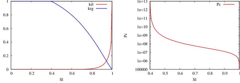
Figure 1: Left: relative permeabilities of the gas and liquid phase  $k_r^\alpha$ ,  $\alpha \in \mathcal{P}$  function of the liquid saturation  $S^l$ . Right: capillary pressure  $P_c$  (in Pa) function of  $S^l$ .
