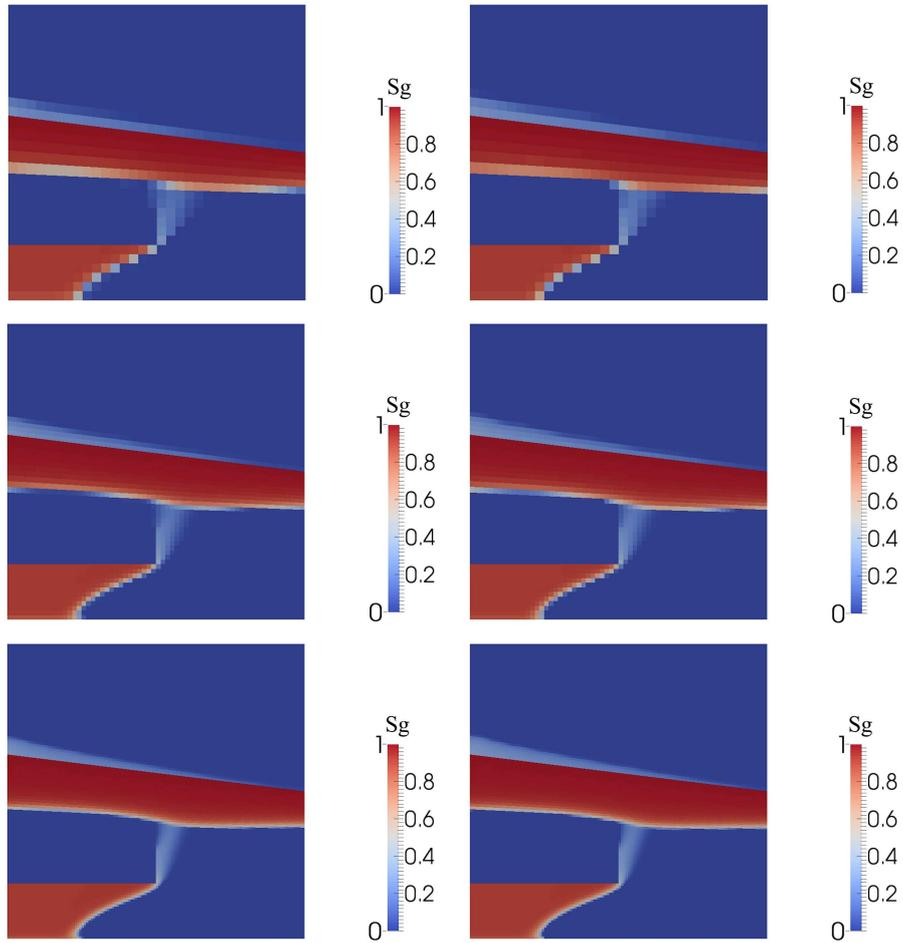
Figure 15: Gas saturation  $S^g$  above the threshold  $10^{-6}$  at final time for the PPF (left) and PSF (right) formulations on the meshes  $32 \times 1 \times 32$ ,  $64 \times 1 \times 64$ ,  $128 \times 1 \times 128$  of the 2D basin.
