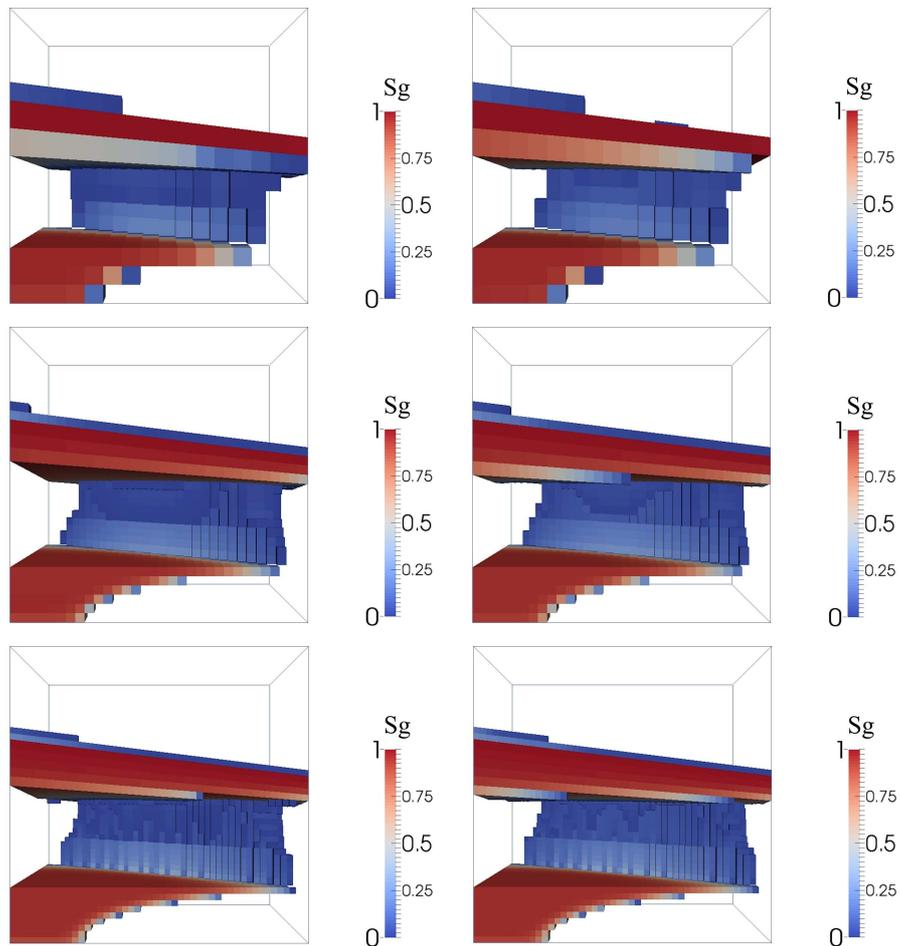
Figure 18: Gas saturation  $S^g$  above the threshold  $10^{-6}$  at final time for the PPF (left) and PSF (right) formulations on the meshes  $16 \times 16 \times 16$ ,  $32 \times 32 \times 32$ ,  $48 \times 48 \times 48$  of the 3D basin.
