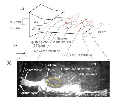
FIG. 1. (a) Schematic of the planar air-water mixing layer from the experimental set-up at LEGI. (b) Airborne smoke particles and a strong LASER sheet are used to observe 2D structures, namely, the liquid film and the recirculation zone downstream of the wave (see Movie 2 of the supplementary material<sup>49</sup> for more details).
