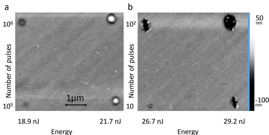
Fig. 5. (a) - (b) AFM images after 10 min in KOH respectively of nano-craters revealed after wet surface etching ( $10^5$  and  $10^6$  pulses @ 18.9 nJ) and nano-hills for  $10^5$  and  $10^6$  pulses with energies 21.7 nJ per pulse; nano-hill (10 pulses, 26.7 nJ per pulse) and polarisation dependent ablation at energies of 26.7 and 29.2 nJ with 10 and  $10^2$  pulses.
