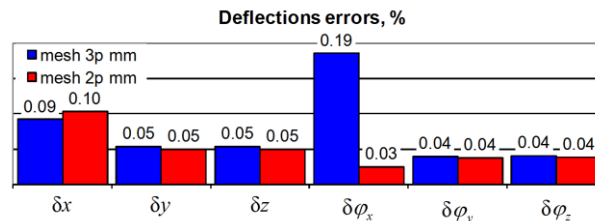
Figure 11 Influence of the stiffness matrix errors on the position accuracy
