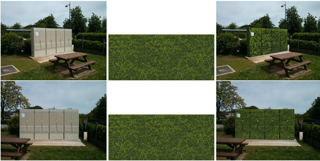
Figure 6: SCOTT makes the visual pollution much less salient. In a concrete case of applying a SCOTT-synthesized concealment texture (middle column), a realistic simulation makes any big “pollutant” (left column) much less salient by giving it an aesthetically more pleasing look (right column).
