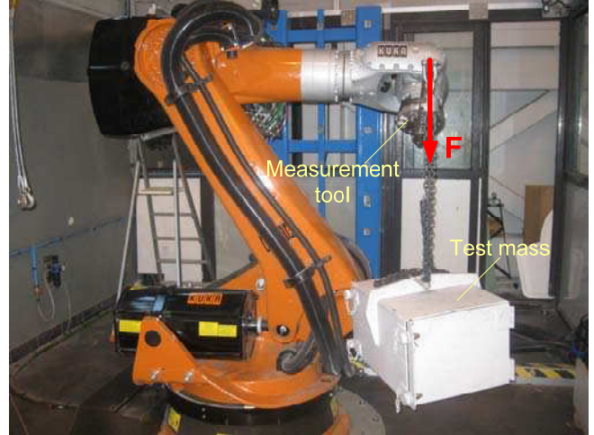
Figure 3. Experimental setup for the identification of the elastostatic parameters
