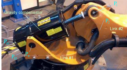
Fig. 1. Gravity compensator of robot KUKA KR-270 TM
