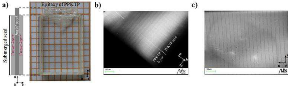
Fig. 4. Periodically domain-structured-KTP films grown on a PPKTP in a flux with the composition 0.1 KTP – 0.6 KPO 3 – 0.3 KF. a) Picture of a PPKTP crystal and the corresponding orientation used for the growth. b) SEM image along the b axis of the grown layer and seed. c) SEM image along the c axis of the grown layer at 225 \mu\text{m} far from the surface of one side of the seed.
