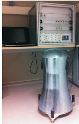
Fig. 16. – \mu QuaS commercial absolute quantum gravimeter. Photo courtesy of P. Bouyer.
