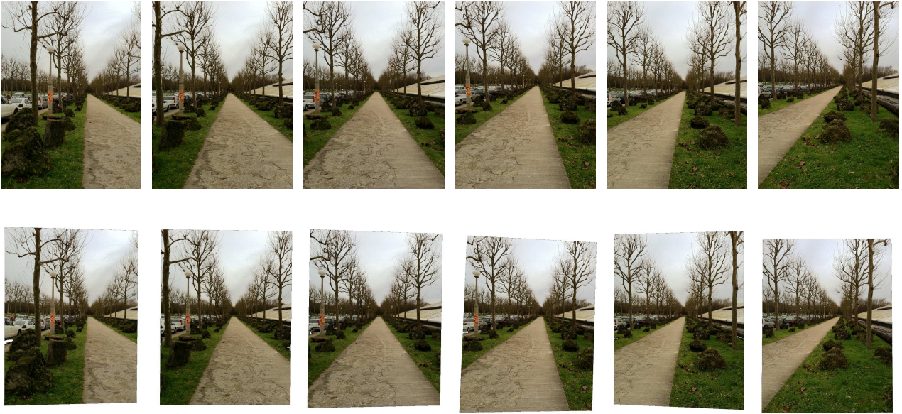
Fig. 9 Multiple image rectification : (Up) six input images. (Down) the six rectified images.
