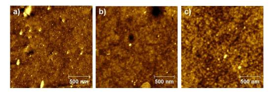
**Figure 2. IC-**AFM height images (2  $\mu$ m x 2  $\mu$ m) of (a) PVC, (b) PVC-NCS and (c) PVC-Lam822, acquired in intermittent contact mode. The height scale was 10 nm for the 3 images.
