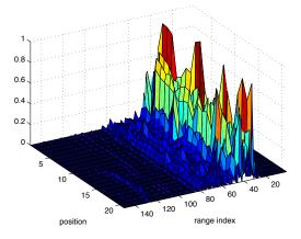
Figure 9. Recovery by full-sampling (1001 frequency points), MF+SBL, estimated noise factor is  $0.5 \times 10^{-1}$ . Due to non-ideal noise estimation the performance is moderate
