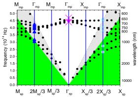
Fig.9 : Band diagram of the single pattern unit cell 2D PhC membrane. At  $\Gamma_{sp}$  point, the coupling mode enhancing the absorption is represented by a purple dot and the non coupling modes by purple crosses. In  $2M_{sp}/3$  the modes are depicted by blue triangles, in  $2X_{sp}/3$  the modes are depicted by light blue hollow circles. The light cone corresponding to the substrate is in light grey hatched pattern, the one corresponding to the air is in plain green.
