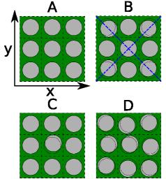
Fig.2 :  $3a \times 3a$  2D PhC. A: Single pattern unit cell PhC used as a reference, B to D: Multiple pattern super cells with symmetric perturbation (diagonals directions represented by the blue dashed lines) (B), with non-symmetric perturbation (shift along  $60^{\circ}$  angle) (C),and with pseudo-disordered perturbation (D). The contours of the unperturbed holes are depicted with the black dashed lines.
