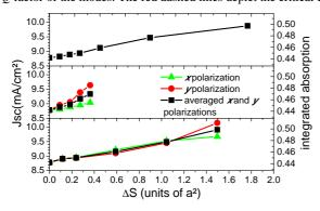
Fig.6 : Short-circuit current density and integrated absorption calculated for different magnitudes of the perturbation and for the 3 different kinds of perturbation: (top) symmetric, (middle) non-symmetric, and (bottom) pseudo-disordered perturbations.
