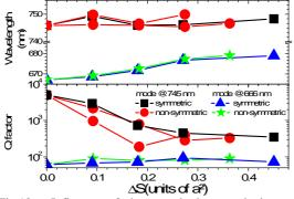
Fig.12 : Influence of the magnitude perturbation on the resonant wavelength (top) and on the quality factor (bottom) of the degenerate modes previously in  $\Gamma$  (around 666 nm) for the symmetric (black square marks) and non-symmetric (red dots) perturbations and in  $2M_{sp}/3$  (around 745 nm) for the symmetric (blue triangles) and non-symmetric (green stars) perturbations.
