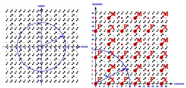
Fig.10. General representation of he reciprocal lattice space, with circle corresponding to the  $|k_{l/l}|$  at a given frequency  $f_{eq}$  (left); Superimposition of two reciprocal lattices, corresponding to a a periodic PhC (red, big dots) and a n.a periodic PhC (black, small dots). n = 3 on this example (right).
