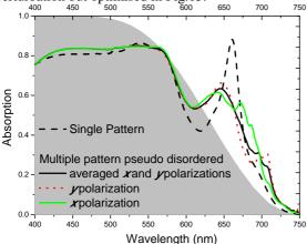
Fig.13: Absorption spectrum for the optimised single pattern in dashed black (a=345 nm, ff=50%) compared to the pseudo disordered structure (average of the two polarizations in black, y polarization in dotted red, x polarization in green (grey)). The absorption spectrum obtained with a Lambertian model is also depicted by the grey background
