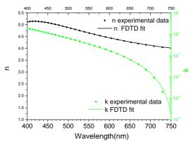
Fig.14 : Measured and fitted optical indices of the a-Si:H layer  $% \left[ {{\left[ {{{\rm{B}}_{\rm{B}}} \right]}_{\rm{A}}} \right]_{\rm{A}}} \right]$
