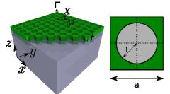
Fig.1 : (Left) Patterned a-Si:H layer ( $C_{4\nu}$  symmetry) on its silica substrate, with in-plane (X, M) and vertical ( $\Gamma$ ) crystallographic directions of the structure. (Right) Top view of a single pattern unit cell, with a period *a* and a radius *r*
