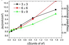
Fig.8 : Short-circuit current density and integrated absorption versus magnitude of the perturbation for the 3 sizes of the super cell:  $3 \times 3$  in black,  $6 \times 6$  in red, and  $9 \times 9$  in green.
