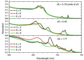
Fig.7 : Absorption spectra for different magnitudes of perturbation for 3 sizes of the super cell:  $3 \times 3$  in black lines with crosses,  $6 \times 6$  in red, and  $9 \times 9$  in green (grey).
