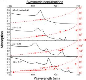
Fig.4 : Absorption spectra for various magnitudes of symmetric perturbation, as depicted in Fig.2B, in black line, left axis. Q factors of the modes, in red dots, right axis. The red dashed line depicts the critical coupling values.
