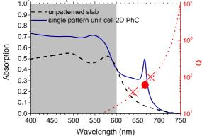
Fig.3 : Absorption spectrum of a single mode, single pattern unit cell 2D PhC membrane (a=220 nm, ff=50%) in blue, compared to the one of the non structured layer in dashed black. In red dotted line, with scale on the right,  $Q_c$  calculated from equation (4), in red dot the Q of the mode at around 666 nm, in red crosses the Q of the non coupling modes found by dipole excitation simulations. The spectral range of interest lies above 600 nm.
