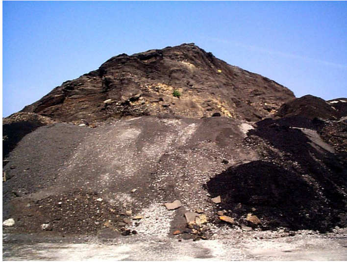
Figure 2. Reclaimed Asphalt Pavement (RAP), stockpile of Blois.
