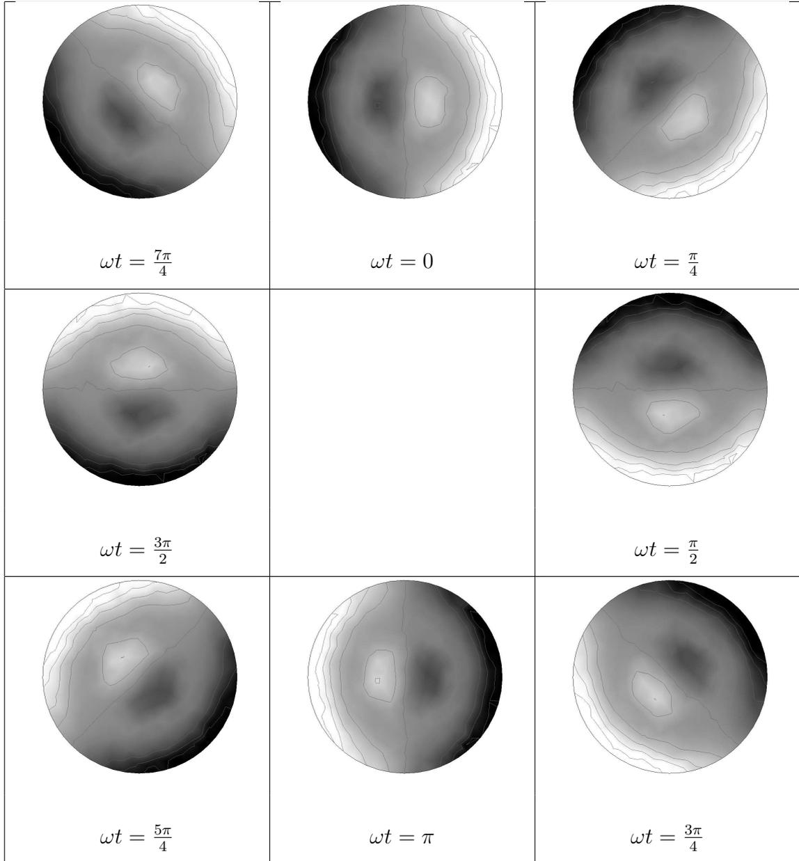
Fig. 16. Velocity fluctuations induced by the rotating mode at the burner outlet.
