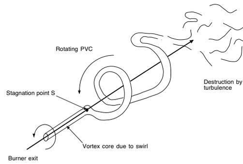
Fig. 1. Schematic representation of a generic PVC.
