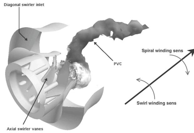
Fig. 11. Visualisation of the PVC in the LES by a pressure iso-surface.
