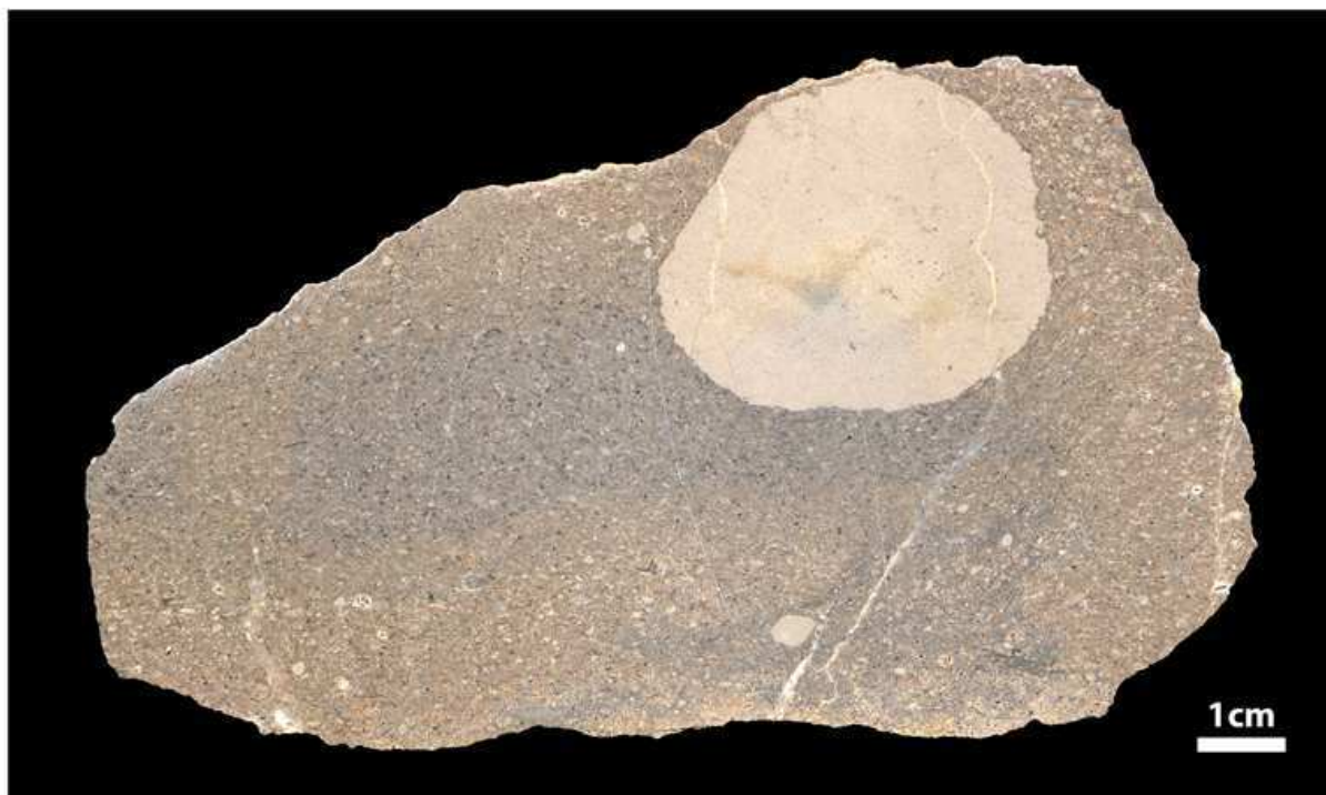
Figure 5: rounded mudstone pebble (intraclast) floating in a bioclastic grainy matrix at level 194.5.
