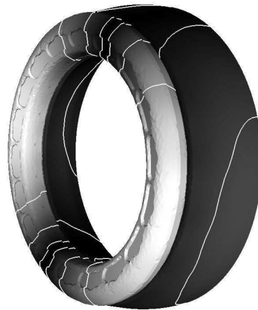
d: First orthoradial/first longitudinal mode - f = 896 Hz
