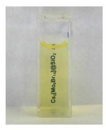
Figure 2. Photography of a  $Cs_2[Mo_6Br_{14}]@SiO_2$  colloid in water (mass concentration ~ 10 g/L).
