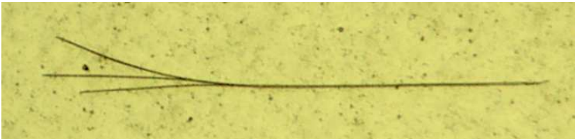
Figure 28: Branching, length of the picture: 0,77 mm.
