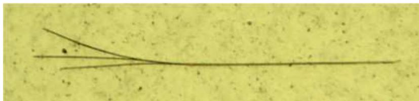
Figure 28: Branching, length of the picture: 0,77 mm.
