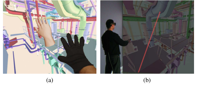
Figure 1: Object selection using different metaphors and devices: (a) Virtual Hand, (b) virtual pointing through a hand-held spatial input device.
