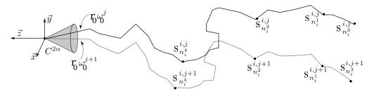
Figure 2: Description of MC-SOME method. In this example, the grey path is a rotation of the black one with respect to its initial direction  $\omega_0^{j+1}$  and M=4.
