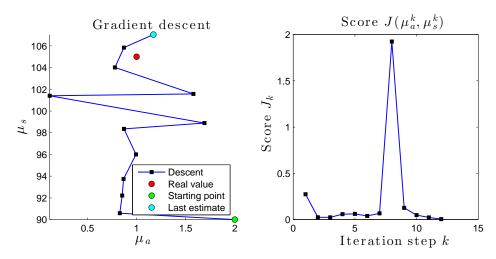
Figure 11: Parameters estimation with an adaptation of Levenberg-Marquardt descent algorithm. The real value of  $(\mu_a^*, \mu_s^*)$  is (1, 105). The starting point is (2, 90). The final estimate is (1.17, 107.04) with a score equal to J = 0.0048.
