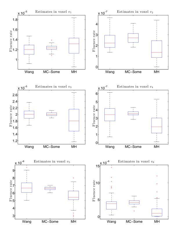
Figure 7: Boxplots of 50 fluence rate estimates in the voxels  $(v_i)_{i=1,\dots,6}$  with WANG, MC-SOME and MH.
