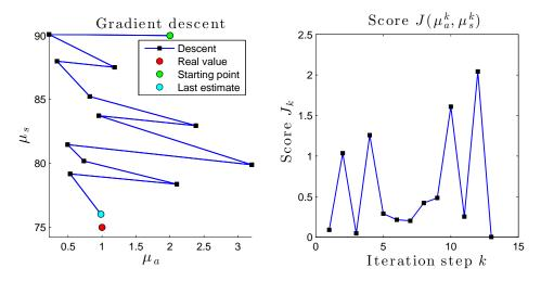
Figure 10: Parameters estimation with an adaptation of Levenberg-Marquardt descent algorithm. The real value of  $(\mu_a^*, \mu_s^*)$  is (1,75). The starting point is (2,90). The final estimate is (1.07,76.02) with a score equal to J = 0.0035.
