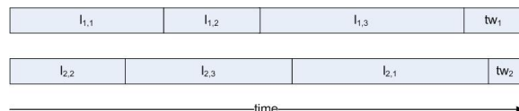
Figure 6. The case k=3, P \geq 4 . Packet rearrangement when l_{1,1}+l_{1,2} \leq l_{2,2}+l_{2,3} . No path reassignment has been performed, yet.
