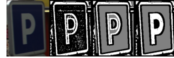
Figure 5: From left to right: 1. Original image, 2. Binarization (function s from eq. 4), 3. Homogeneity constraint (eq. 5), 4. Filling in small homogeneous regions.
