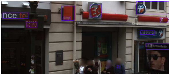
Figure 9: The system localizes correctly text in the image (even with rotated text) but it detects aligned windows as text.
