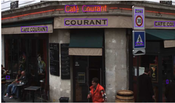
Figure 10: Text is correctly localized, but the classification step fails on the end of the word courant in red and zebra crossing sign is seen as text.
