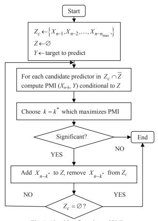
Fig. 1. Algorithm flow chart of PMI
