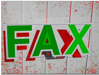
Fig. 15 Result of the grouping process: a bounding box is surrounding the detected text region.
