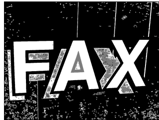
Fig. 9 Geometrical filter result on the FAX segmented image. Black regions are dismissed, white regions are letter candidates for classification step.
