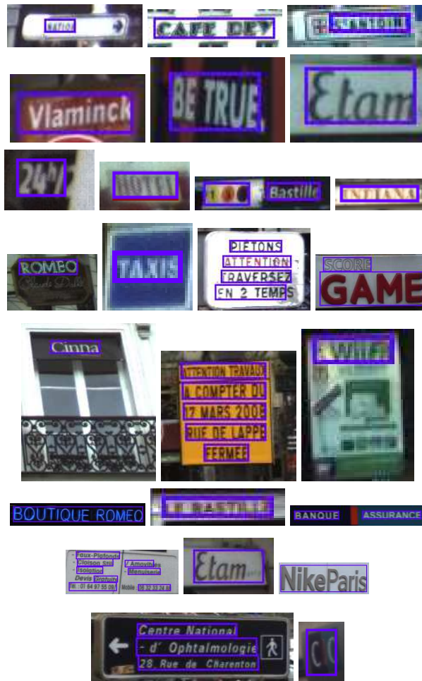
Fig. 24 Examples of text boxes from many different ITOWNS images detected by our system.
