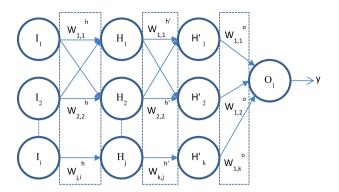
Fig. 10 – Example of a multi-layer feed-forward neural network [38]. I: inputs, H and H': hidden neurons, O: output neurons,  $W_{j,l}^{h}$ : weights between hidden neuron j and input I,  $W_{k,j}^{h'}$ : weights between hidden neuron j and hidden neuron k,  $W_{m,k}^{o}$ : weights between hidden neuron k and output neuron m.
