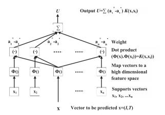
Fig. 11 – Illustration of a SVM PEMFC model, with inputscurrent density I and temperature T, and output-voltage U. Support vectors and weights are decided during training. [Zhong, Z.-D. et al. (2006)] [55].
