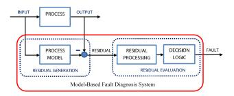
Fig. 1 – Model-based fault diagnosis scheme [Ding SX (2008)] [6].
