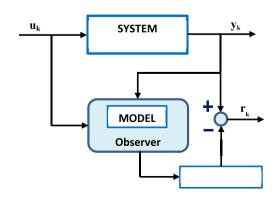
Fig. 8 – Observer-based residual generator scheme [Witczak, M. (2003)] [31].
