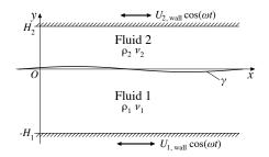
FIGURE 10. Two-layer oscillatory flows with bounding walls
