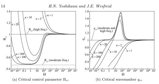
FIGURE 4. Values of the control parameter B and the most unstable mode q on the instability threshold for different viscosity contrast values. The density contrast  $\rho$  is 0.9 for all the curves.
