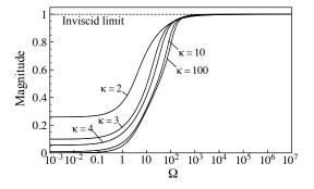
FIGURE 5. Magnitude of the phase velocity of waves in the interface reference frame, at the instability threshold. Magnitude is normalized by the magnitude in the inviscid limit. ( $\rho = 0.9$  for all the curves.)
