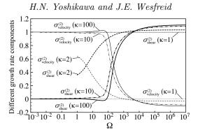
FIGURE 7. Different components of the third order growth rate  $\sigma^{(2)}$  at the instability threshold. Both velocity- and shear-induced contributions,  $\sigma^{(2)}_{\text{velocity}}$  and  $\sigma^{(2)}_{\text{shear}}$ , are shown for different viscosity contrasts  $\kappa$  after normalization by the capillary-gravity contribution  $|\sigma^{(2)}_{-}|$ . ( $\rho = 0.9$  for all the curves.)
