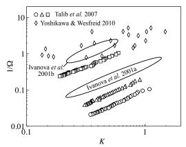
FIGURE 2. Parameter ranges of existing experiments. The inviscid theory for small amplitude oscillatory flows (1.1) is valid in the limit of  $K \to 0$  and  $1/\Omega \to 0$ .
