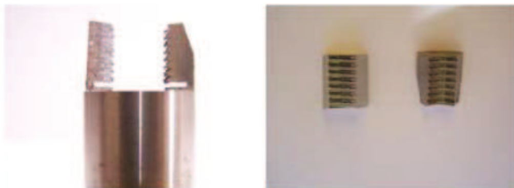
Figure 3. The cut parts of formed threads. 137x49mm (96 x 96 DPI)
