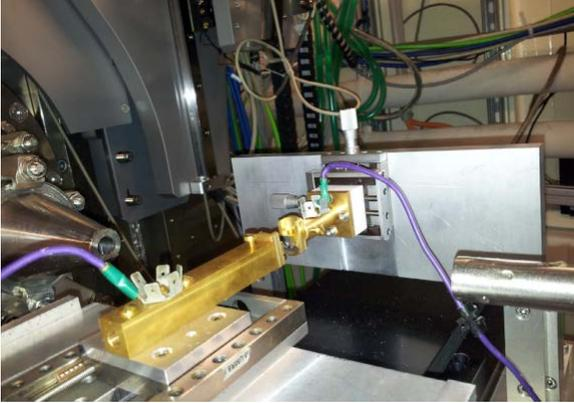
Fig. 1: Photo of the experimental apparatus mounted on the Swing beamline at the Soleil synchrotron in Saclay, France. X-rays exit the beamline through the tube on the right, pass through the inter-electrode gap (through the arc when it is lit) and enter the detector chamber through the cone on the left. The detector is located inside a 10 meter long evacuated chamber (left in the picture) and set at 4.075 m from the arc center.
