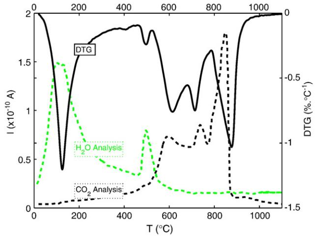
Fig. 4. DTG data and results of mass spectroscopy (ion currents for  $\text{H}_2\text{O}$  and  $\text{CO}_2$ ) determined in a 2 mm-deep sample (T1) of the cement paste P45 after 14 days of accelerated carbonation.
