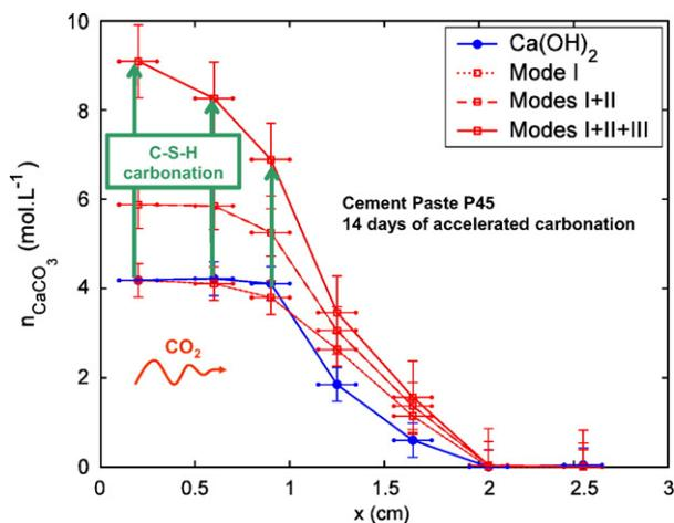
Fig. 5.  $\text{CaCO}_3$  profiles for the cement paste P45 after 14 days of accelerated carbonation. Profiles corresponding to  $\text{CaCO}_3$  produced by the sole carbonation of  $\text{Ca}(\text{OH})_2$  and to the three DTG modes of  $\text{CaCO}_3$  decomposition.
