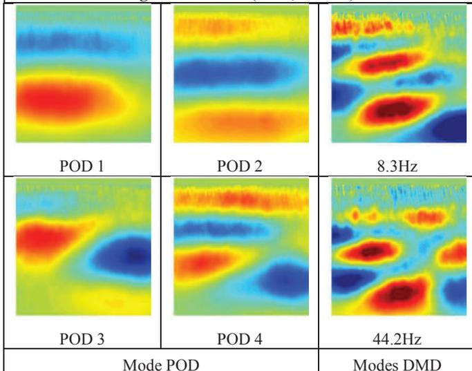
Figure 13 – Modes ( $\sigma = 1.5, \alpha = 10^\circ$ )
