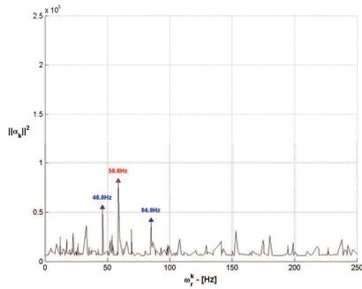
Figure 8 – Spectre de modes ( $\sigma = 2, \alpha = 10^\circ$ )
