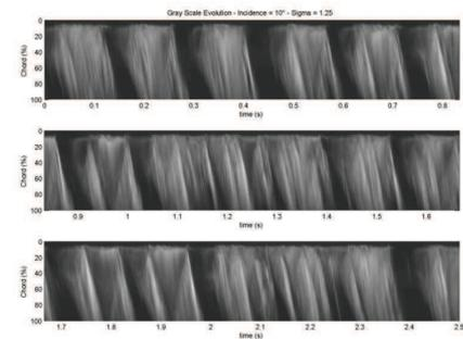
Figure 7 – Diagramme spatio-temporel ( $\sigma = 1.25, \alpha = 10^\circ$ )
