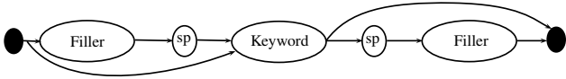
Fig. 1. Global line model containing the keyword, and the filler model. The line model is also made of a space model ("SP"), and structural initial and final models.
