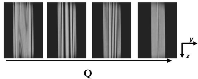
FIG. 3. Monochromatic light interference at the thin film in the Plateau border regime (Fig. 2), viewed from the *side* ( $x$ -direction in Fig. 1). Complex swirling motion is only seen at very low flow rates  $Q$ , while a laminar flow is found over the whole range of  $Q$  applied for the measurements presented in this article.
