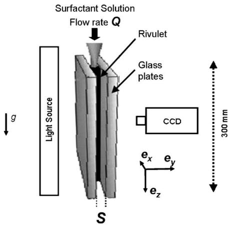
FIG. 1. Sketch of the setup: surfactant solution is injected at constant flow rate  $Q$  between the two narrowly spaced, vertical glass plates. The liquid descends under gravity and forms a *rivulet*, which is straight and vertical at sufficiently low flow rates.
