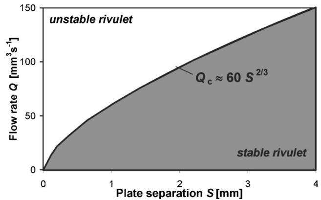
FIG. 13. The rivulet is unstable above a critical flow rate, which depends on the plate separation  $S$ . Shown here is the experimentally established stability diagram for commercial Fairy Liquid solutions [Eq. (23), Ref. 1]. All our experiments are conducted in the stable (gray) zone.
