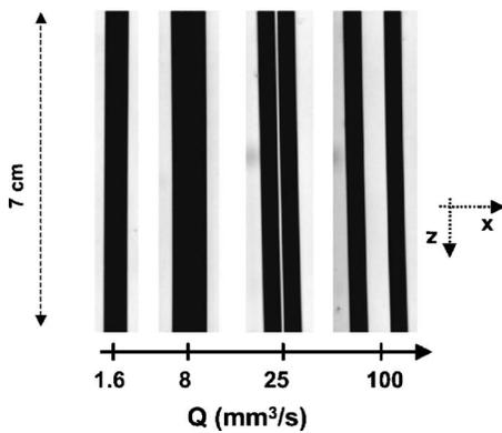
FIG. 14. Typical images of the rivulet for increasing flow rate  $Q$ . The two left images correspond to the Plateau border regime (left-hand side of Fig. 2), while the two right images are in the liquid bridge regime (right-hand side of Fig. 2).
