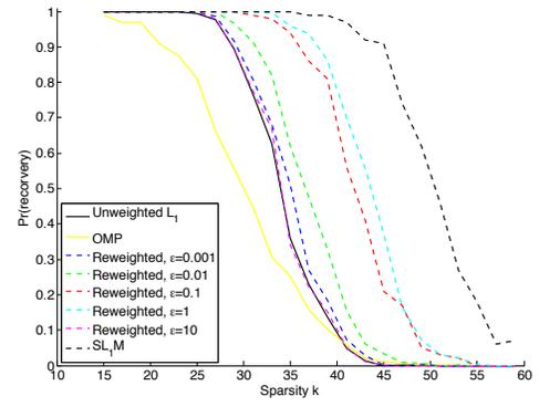
Fig. 1. Empirical probability of successful recovery versus the sparsity level  $k$  for the OMP method [11], the classical reweighting of [3] with various  $\epsilon$  and the proposed one ( $S\ell_1M$ ).
