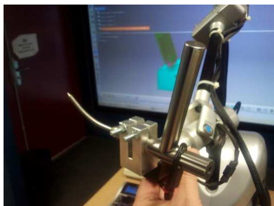
Fig. 3. The instrument tightened by the piece is tied to the haptic arm
