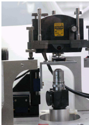
Fig. 10. AFM with substrate in liquid medium.
