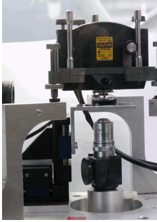
Fig. 10. AFM with substrate in liquid medium.
