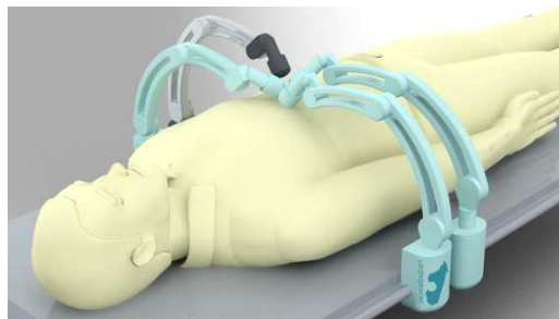
Fig. 1: Robot-assisted magnetic manipulation with several mobile coils.
