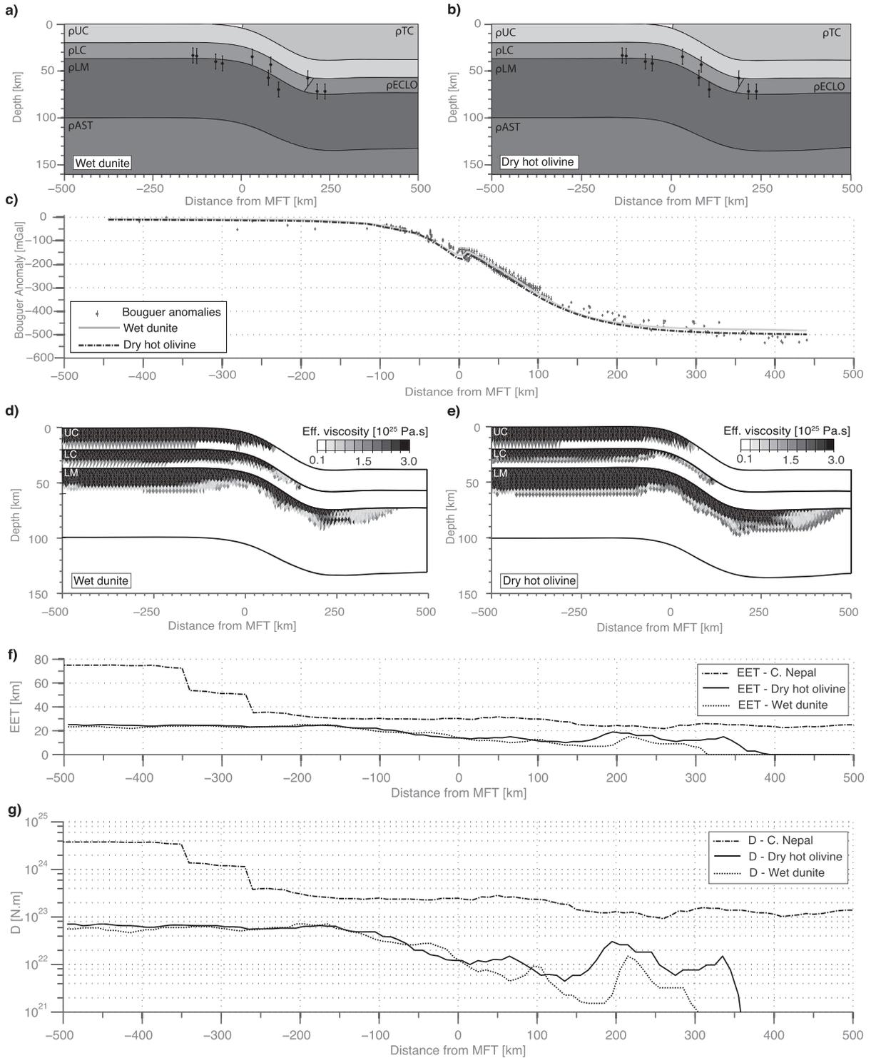
**Figure 3.** Preferred model results. (a, b) Resulting geometry with projected seismic Moho depths (dots with error bars) and density structure. Densities as in Table S1 and  $\rho_{ECLO} = 3050 \text{ kg m}^{-3}$ . (c) Synthetic (lines) and observed Bouguer anomalies (dots with error bars). (d, e) Effective viscosity profiles. (f, g) Effective elastic thickness and flexural rigidity of the preferred models and of the Nepali model (Berthet et al., submitted manuscript, 2013) for comparison.
